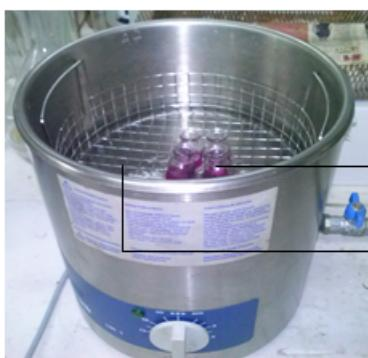
Fig. 3. Experimental setup for indirect sonication
