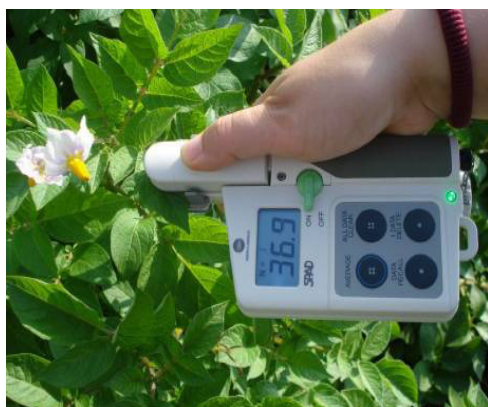
Fig.7 Monitoring the leaf chlorophyll content of potato crop with SPAD 502
