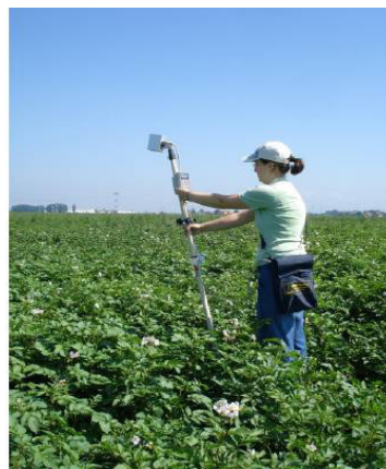
Fig.8 Monitoring the the reflectance of potato crop with CropScan
