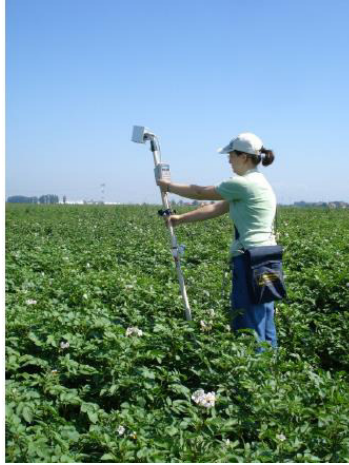
Fig. 18. Monitoring the reflectance of potato crop with CROPSCAN multispectral radiometer
