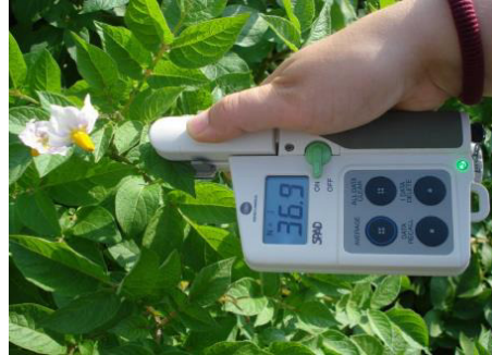
Fig. 17. Monitoring the leaf chlorophyll content of potato crop with SPAD 502
