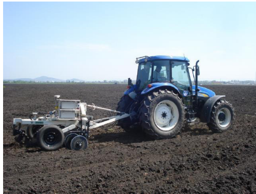
Fig. 11. Soil electrical conductivity monitoring with VERIS (Mobile Sensor Platform)
