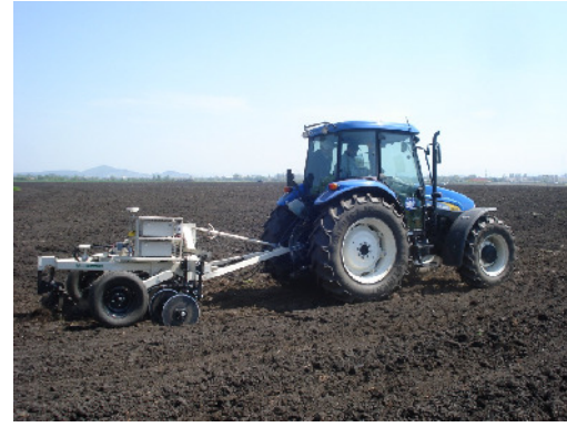
Fig. 2. Soil electrical conductivity monitoring with VERIS (Mobile Sensor Platform)
